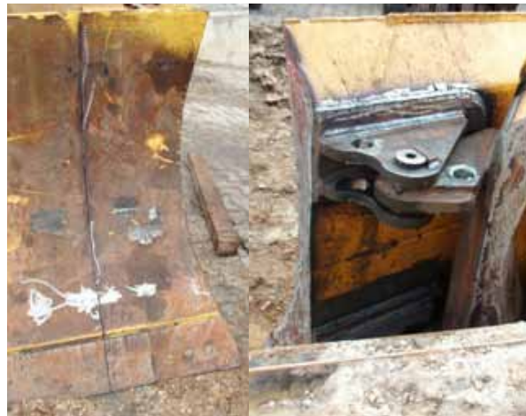
Bulldozer blade conversion on folding shield
