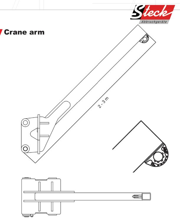
In a few minutes every excavator can be equipped with a KTH crane arm. This combination is helpful for internal and external loading and unloading activities.
