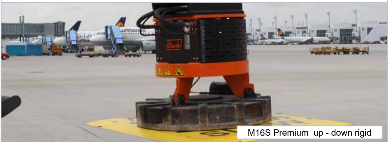
Magnetic plate with teeth
